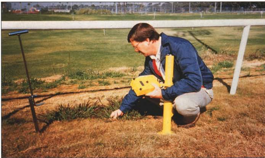
The author measures turf hardness with a Clegg Impact Hammer at Hollywood Park Race Track.
