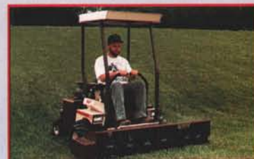
40- or 60-inch AERA-vator™ penetrates hard, dry soil without irrigation. ROPS with overhead canopy is optional.
