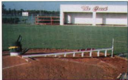
The purpose of Perry's "gadgets" — such as this device for setting mound blocks in high stress areas — is to make turf managers' jobs easier and playing surfaces safer.
