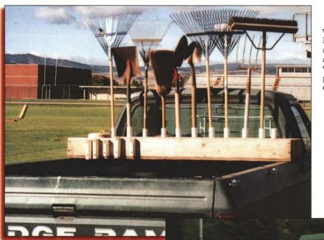
Be innovative with homemade equipment wagons that save steps, labor and duplication of responsibilities. "Neat and efficient" means to transport tools and still have the bed open.
