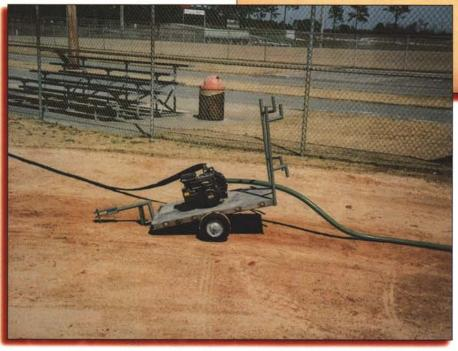
Eliminate certain traditions and create easier means of doing a trivial task like removing water from turf and clay with a movable sump pump.
