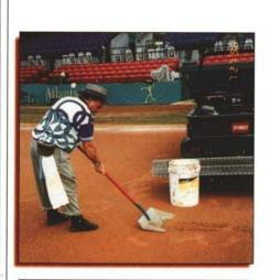
Remove debris, stones and larger size particles while saving infield material and calcined clay. A soilsifter is a 21st century tool.
