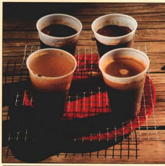
Cup test for performance of skinned area soil samples.
