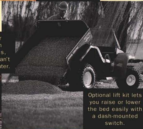
Optional lift kit lets you raise or lower the bed easily with a dash-mounted switch.
