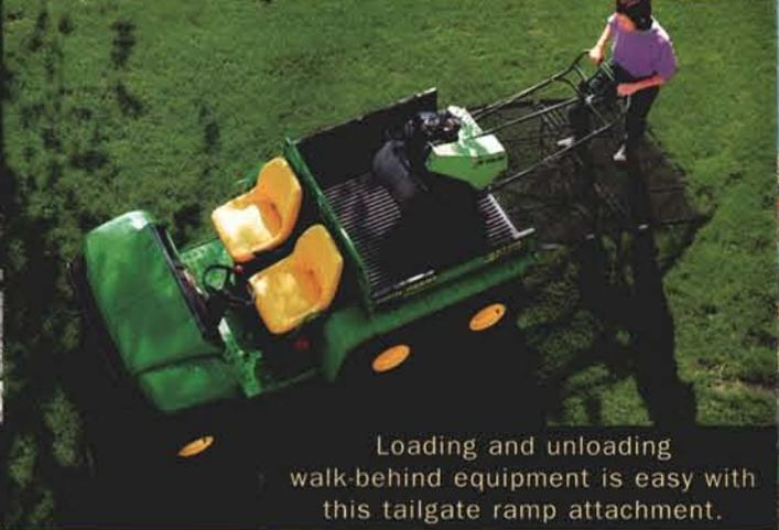
Loading and unloading walk-behind equipment is easy with this tailgate ramp attachment.
