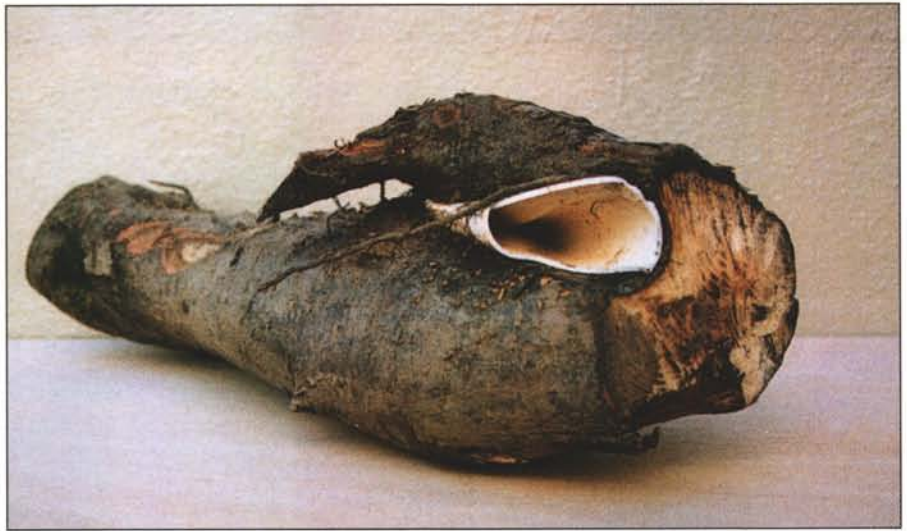
Avoid laying PVC pipe close to the trunks of trees, which can crush pipe.
