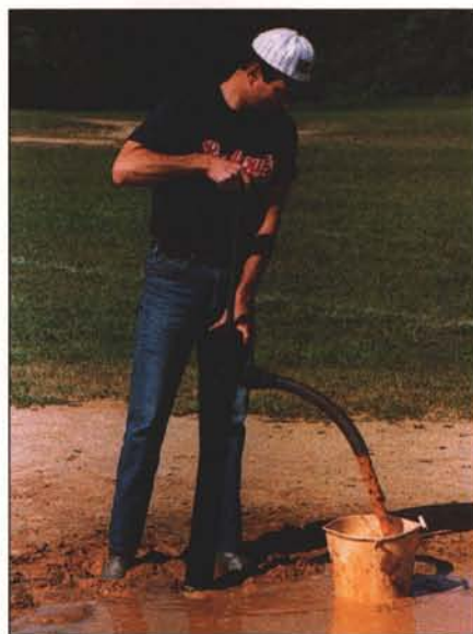
Hand pumps (or small gas-powered pumps) work in puddles one to two inches deep or deeper and can drain water into a turf area, a bucket or a cart. Photo courtesy: Kuranda U.S.A.
