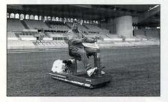
The Stadium Roller 7000, by Wood Bay Enterprises of Las Vegas, NV, features a three-roller configuration comprised of one non-slip drive roller and two steering rollers. With a 5.5-hp Honda engine and a Snow-Nebstead power transmission, the roller utilizes a hand throttle for increased safety and ease. The roller travels at approximately seven miles per hour.
