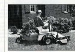
Grasshopper's new model 725K zeroradius outfront mower, with its 25-hp Kohler Command V-Twin OHV engine, is the company's largest air-cooled unit.
