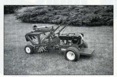
Terracare's 1997 Riding Aerator allows the operator to aerate one acre per hour with ease. The 98-tine aerator is 22 inches wide and produces a 3 1/2 inch by 4 1/4 inch pattern. Equipped with an eight-hp electric start Briggs & Stratton engine, it features hydrostatic drive with an electric screw jack for lifting the tines in and out of the ground.
