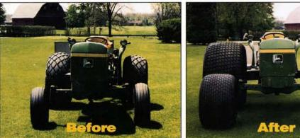
• Top Dressing • Spraying • Mowing • Back Filling Traps • Aerating The large contact area of the flotation tire effectively distributes load over a broad area. This produces lower unit ground pressure resulting in minimized soil compaction.
