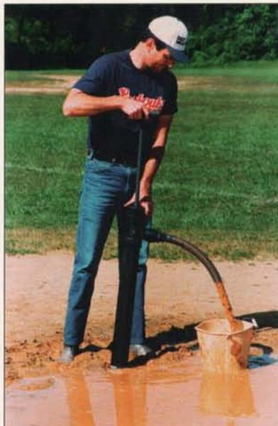
The Diamond Pump is a durable, non-clogging hand pump which easily removes 18-20 gallons of water per minute from dirt infields, sand traps, ditches. Made of tough ABS and PVC, a six-inch aluminum disc prevents mud from being drawn directly into the pump. Absolutely will not clog.
