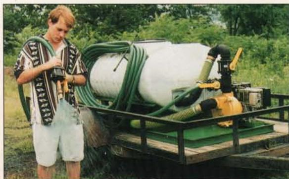
Faster germination and lower labor costs are among the advantages of a *Turbo Turf Hydro Seeding System*. Pictured above is an HS-300E. This unit will apply seed, fertilizer, and mulch in one step. Coverage is 4000 sq. feet per load. Mixing time is under 60 seconds, and application time is 9 minutes. The HS-300-E has a retail price of \$3,995. Other sizes are available from 50 gallons to 1600 gallons. Prices start at \$1,295.
