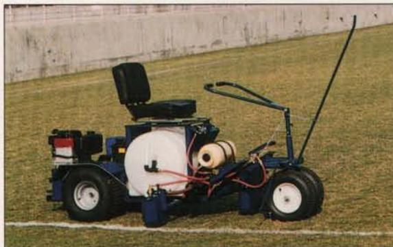
The Jaydee Driver Liner is a self-propelled riding line marker. The 35-gallon paint tank carries enough marking material for a complete game field, or several practice fields. The 2-gallon flush tank cleans the discharge lines for work breaks, travel, or overnight. The center- or side-mark sprayshields are always operator-visible. A nearly zero turning radius reduces or eliminates back-and-turn maneuvers.
