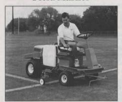
The Top Liner field marker, designed for lining and marking baseball, softball, football, soccer and track meet fields, is engineered to deliver the tight turning and quick power response that are most desirable in athletic field marking. The low-maintenance hydrostatic drive, coupled with an Eaton transaxle, provides smooth and fast performance for marking jobs with a minimum of work time.
