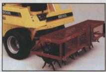
Unique up-front mounted core aerators help grounds managers get more production from their John Deere, Kubota, Ford, and Excel Hustler mowers. Millcreek core plug aerators have a protective safety cage, and individually mounted spoon wheels to allow easier turning without damage to turf. Affordable Millcreek aerators come in wide variety of sizes and styles in addition to the front-mounted units.
