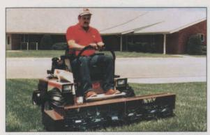
New AERA-vator™ attachment for Grasshopper zero-radius outfront mowers aerates established turf or prepares bare ground for seeding or sodding. Forged steel tines vibrate rapidly to penetrate and fracture the hardest, dryest soils without leaving unsightly plugs. Quik-D-Tatch® mounting system lets you switch quickly from Combo Mulching™ Deck to attachments.
