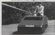
The Water Hog is the world's first surface water removal system with an ability to pump more than 6,000 gallons per hour from turf or hard surfaces. It doesn't just push water from one place to another. It picks it up and gets rid of it by shooting it into a waste area as it goes or holding it in tanks to be hauled away and dumped.
