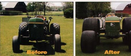
• Top Dressing • Spraying • Mowing • Back Filling Traps • Aerating The large contact area of the flotation tire effectively distributes load over a broad area. This produces lower unit ground pressure resulting in minimized soil compaction.
