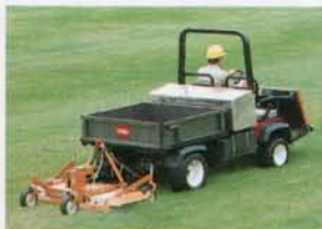
Mowing is a breeze with split bed, 3 pt. hitch & 60" PTO rotary.
