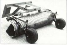
York Rakes builds the models BCF and CSF specifically for use with Bobcat and Case skid-steer loaders, and the model SSF can be used with most other makes.
