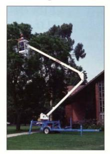
The EAGLE 44. manufactured by AmeriQuip, is a trailer mounted, articulated aerial lift with a 25 ft. side reach and 44 ft. working height. features positive bucket leveling and 360° continuous rotation.
