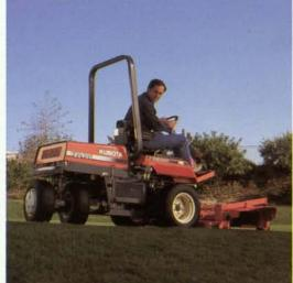
power. Both have Kubota diesel engines, and are equipped with hydrostatic rearwheel power steering for easy handling. A wide selection of Performance Matched Implements provide the versatility. They include triplex reel, rotary, flail and mulching rear discharge mowers, rotary broom, leaf blower, snowblower, and front blade. Roomy operator's deck, tilt steering wheel, and excellent visibility increase comfort and productivity.
