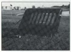
The TORO Submersible Aspirating Aerator aids in the natural aquatic rejuvenation process by increasing dissolved oxygen levels, providing circulation, creating horizontal water flow velocities and maintaining aerobic conditions throughout the water column.
