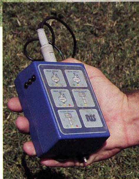
Mark Satterfield, UC Davis irrigation technician, trouble-shoots a wiring problem with an irrigation control wire analyzer. Photos courtesy: Bob Milano. (Inset) Close-up of an irrigation control wire analyzer.
