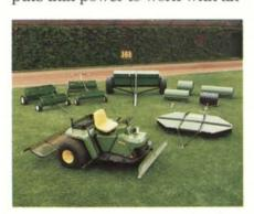
Attachments like spreaders, seeders, rollers, brushes, scarifiers, a wide blade, and field finisher help the 1200 shine on the field.
