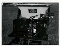
Terracare's skid-mount topdresser will fit on most utility vehicles. It is fully hydraulic, with a variable speed on the feed auger and the spinners. It is powered by an 8-hp Briggs & Stratton engine.
