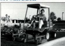
Kubota Tractor Corporation's mulching, rear-discharge mower deck is compatible with Kubota's F2100 and F2400 mowing tractors. It features cutting widths of 60 and 72 inches and three 1-inch-diameter, heavy-duty spindles with two blades per spindle.
