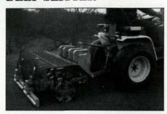
The 4-foot Multislit has five slitting blades fitted to each of eight large diameter plates. The tine plates have a wide rim to reduce marking when working at full penetration. Six- or 8-inch sharpened slitting blades are available for use on fine turf areas such as golf greens, and 6-inch heavy-duty slitting tines are available for outfield turf.
