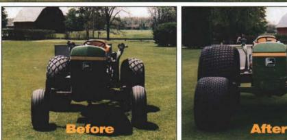
• Top Dressing • Spraying • Mowing • Back Filling Traps • Aerating The large contact area of the flotation tire effectively distributes load over a broad area. This produces lower unit ground pressure resulting in minimized soil compaction.
