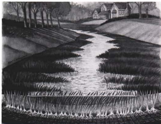
LANDLOK erosion mat
