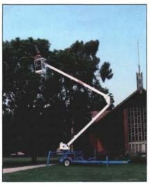
The EAGLE 44, manufactured by AmeriQuip, is a trailer mounted, articulated aerial lift with a 25 ft. side reach and 44 ft. working height.
