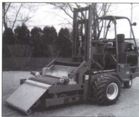
Forklift-attached sod installer from Cygnet Turf & Equipment.
