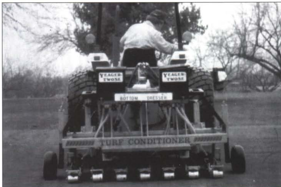
Subsurface polymer planter in action. Photo courtesy Ken Harrison, Hydrosource.
