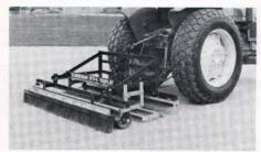
For levelling and restoring hard porous surfaces such as baseball infields and run-
