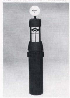
A plug of living sod, not a plastic or metal cover, conceals and protects Hunter's I-44 Sod Cup sprinkler when retracted. It is designed for moderate to high-capacity usage on golf courses, playing fields and other public areas, and has been extensively field-tested at the PGA West Golf Course
