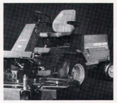
Single-pedal hydrostatic control, standard on the Jaguar 4000, controls the machine's forward and reverse movements. Automatic differential lock is available on two models, and reduces wheel slippage and turf damage.
