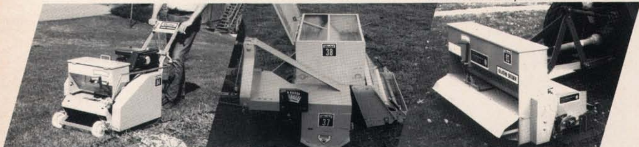
MODEL 84 walk-behind slit seeder, 18 hp, self propelled.
