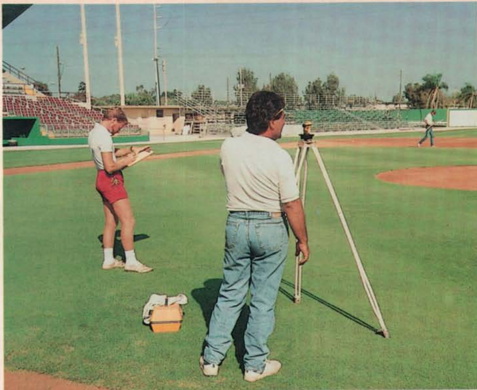
Timpanaro (center) checks infield elevation with transit.
