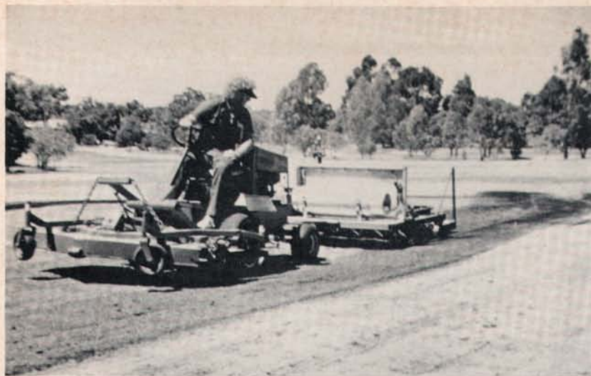
Propane burner used as an experiment to burn off thatch and kill fungi on fairway.
