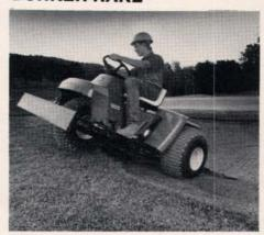
John Deere has introduced the Model 1200 bunker rake for golf course maintenance professionals. The two-wheel-drive unit is powered by a ten-hp, four-cycle Kawasaki engine.
