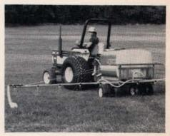
A new foam marker for use with boomtype sprayers has been introduced by Lesco, Inc. The marker, used on large, open turf areas such as golf courses, parks and commercial sites, is designed to prevent costly skips and overlaps when applying chemical products or fertilizers.
