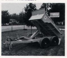
A turf dump trailer specially designed to produce the least possible compaction has been introduced by Holland Equipment Ltd. The Aer-Way dump trailer incorporates a six-point attachment of the hoist for maximum stability.
