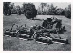
Brouwer transportable PTO-driven mowers are manufactured to give a fine-quality cut even in adverse conditions. The standard mowers, with their fixed mowing units, rugged design and proven mechanical drive, offer reliability and low maintenance costs.
