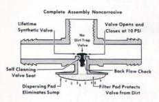
Protect your turf irrigation systems with a King Drain from King Technologies, Inc. The durable, pressure-sensitive valves are molded from PVC or ABS plastic, and are
