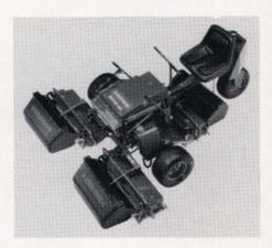
yet cut a 71-inch swath. The TR15B offers an optional three-wheel drive for additional traction and climbing power.
