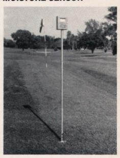
Turf-Tec International has added a moisture sensor to its line of diagnostic tools. This tool adjusts to check moisture at depths from one to six inches in the soil profile.
