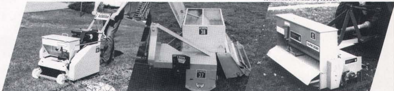
MODEL 84 walk-behind slit seeder, 18 hp, self propelled.
