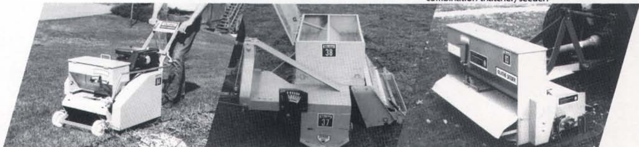
MODEL 84 walk-behind slit seeder, 18 hp, self propelled.
