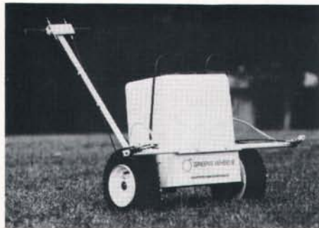
The Greens Wheelie by Wheel Spray Corp., is a liquid chemical spreader with
