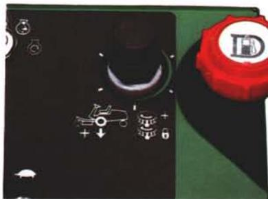
*Standard equipment on the F930 and F935 (optional on the F910, F912, and F915), John Deere's exclusive hydraulic weight transfer valve lets you shift the weight of the deck to the drive wheels for added traction on the go.*
