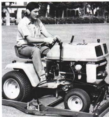
The Haley Planer is a verticutter centered on a six-foot-long frame built for bowling greens.
