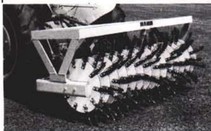
TM-140 Aerifies a six feet swath using your tractor's 3-point hitch.
