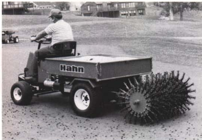
Drum-type aerifiers can be pulled by nearly any type of turf vehicle.
