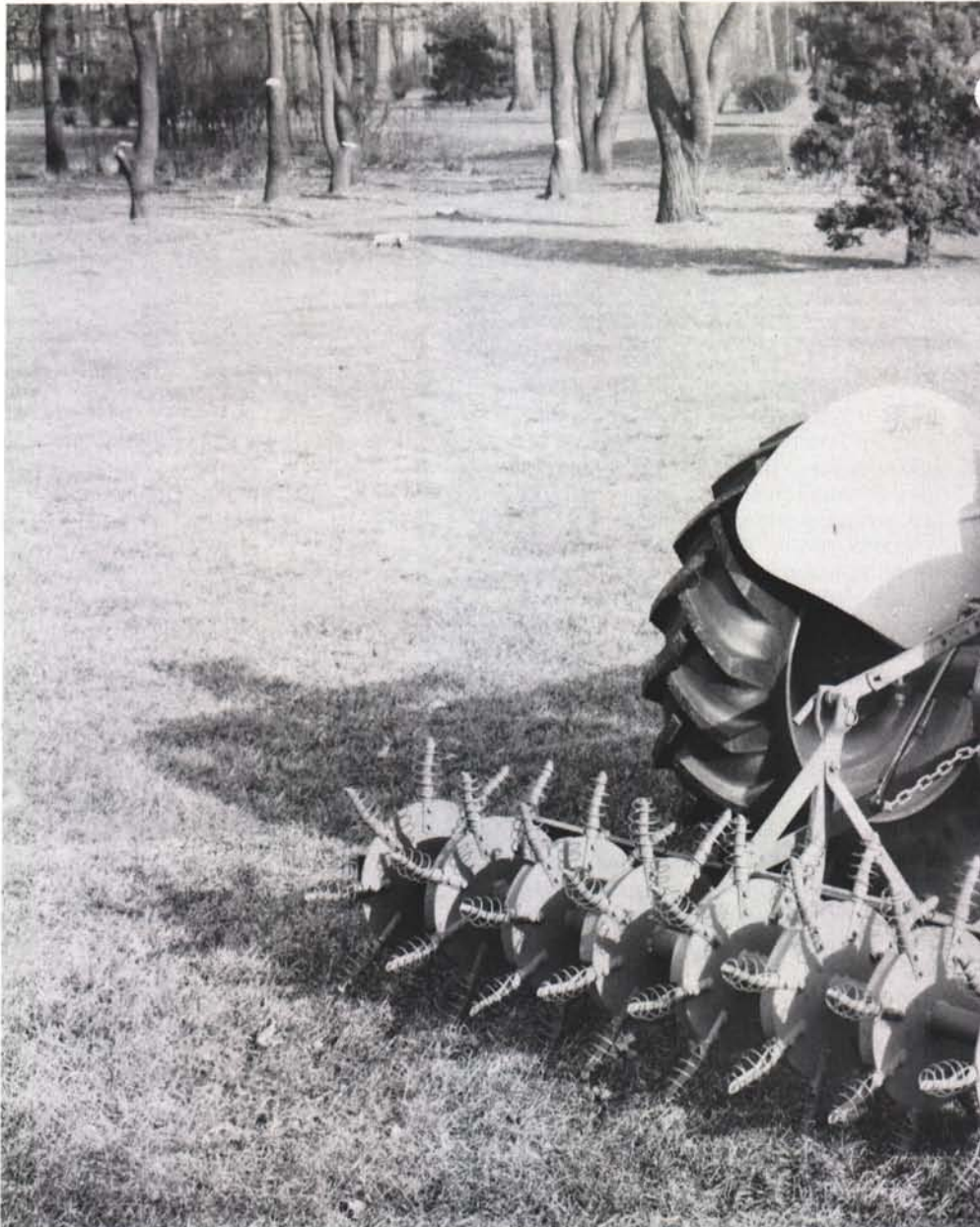
The original West Point spoon-type aerifier being used in a park in 1953. Photo courtesy of Ha
