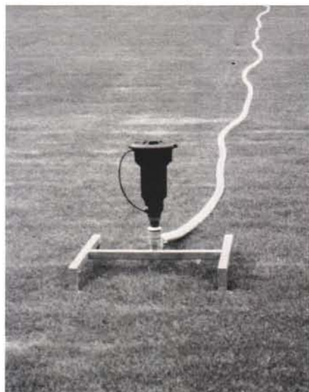
No sprinkler heads are allowed on the field so Tingley rigged up this Toro head on a stand.
