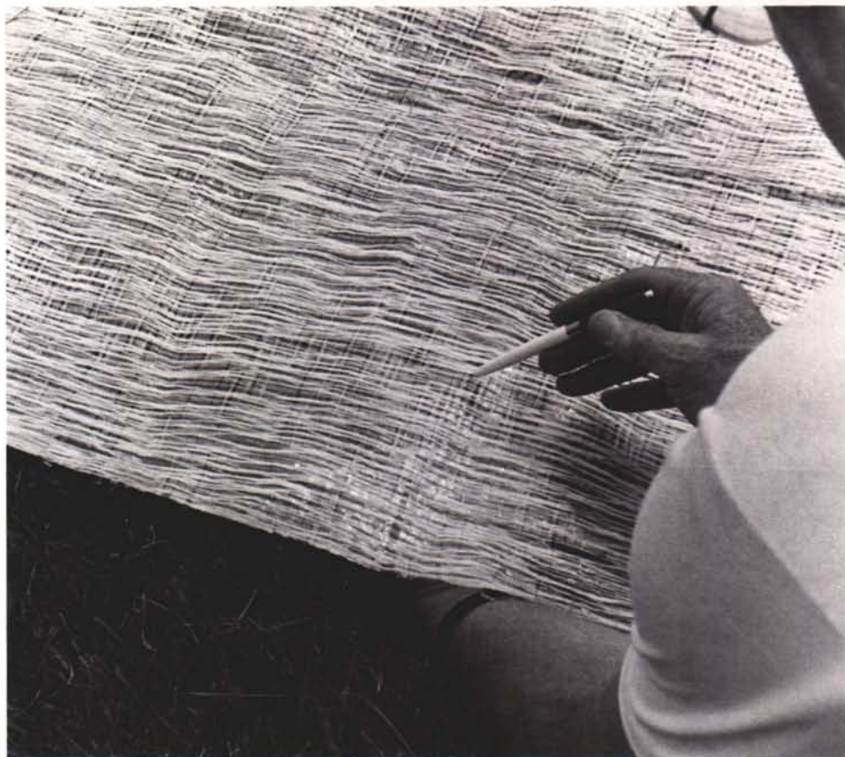
Evergreen protective covers allow 85 percent penetration of sunlight to the turf.
