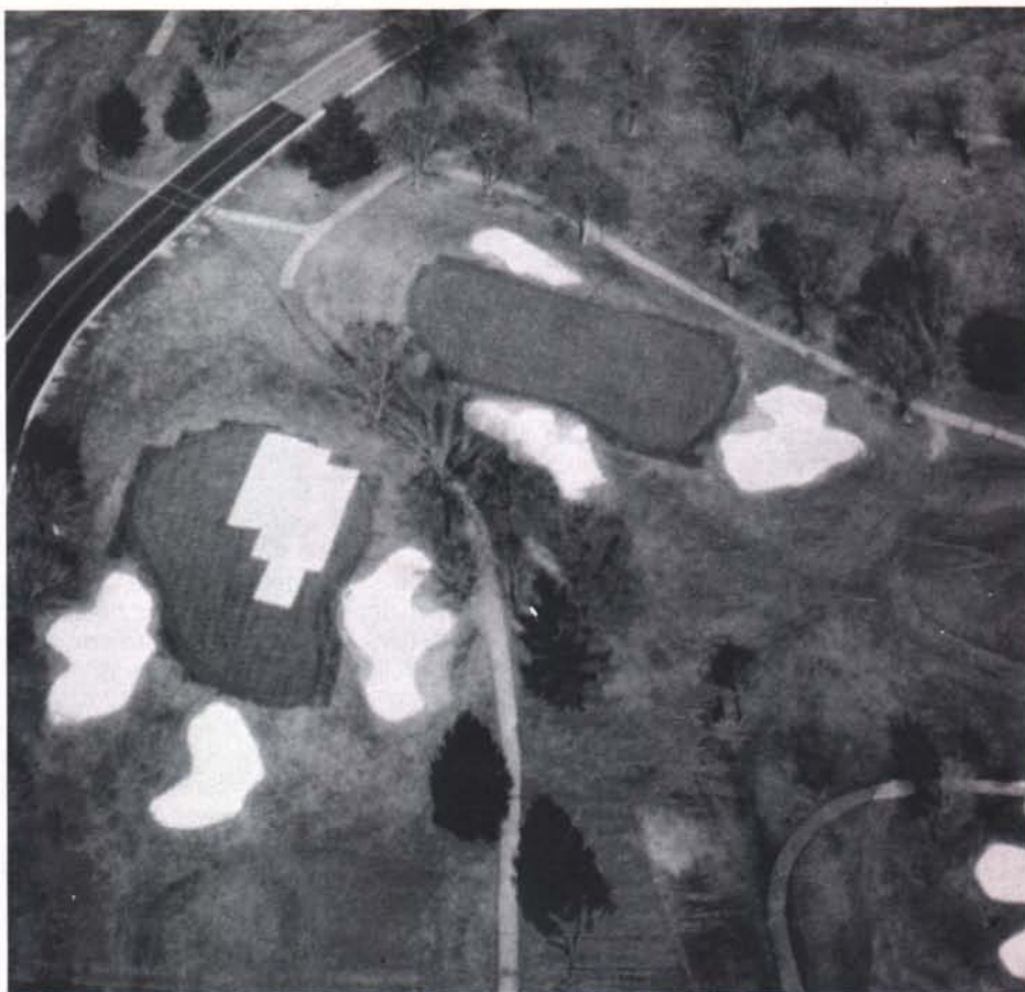
Aerial view of golf course with geotextile warming cover on part of one green.
