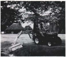
If the park, campus or golf course you maintain has a large amount of sloping roadsides, lake shore area or fences that require labor-intensive hand cutting, the Beaver Flail Cutter can increase your maintenance efficiency. Attached to any 20-35 hp compact tractors with category 1 three-point hitch and 540 r.p.m. PTO, the hydraulic arm and flail mower enable the operator to mow utility turf as far as nine feet from the tractor.
