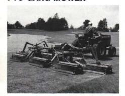
Large-area mowing can still be economical with Brouwer's PTO gang mowers. These transportable mowers can be pulled with small tractors with lower fuel consumption and less weight to cause compaction. The reel units can be lifted for transport manually or with an optional hydraulic lift.
