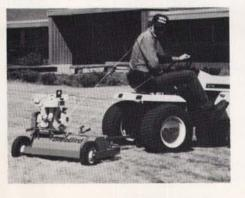
Any riding mower, garden tractor or turf vehicle can tow Bluebird's lawn comber. Fortyeight free-swinging blades of case-hardened steel spin on a flail rotor to cut grass runners and lift out thatch. A locking height adjustment enables professional turf managers to change the cutting depth by minute amounts.
