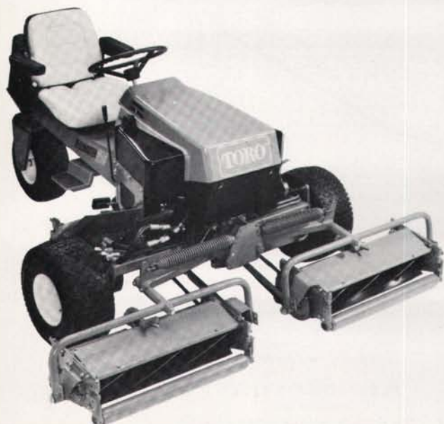
The Toro Reelmaster 216 has a hydrostatic transmission and six-foot cutting width.
