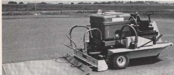
SELF CONTAINED UNIT: Scarifier & Sprayer mounted on the Olathe Turf truck. A complete ATHLETIC FIELD MACHINE!
