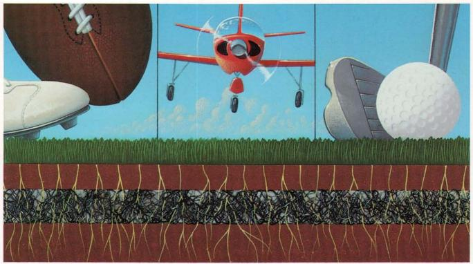
With the Enkaturf system, grass can thrive where it needs to work the hardest. Our black 3-dimensional matting anchors roots and protects them against surface abuse and compaction.
