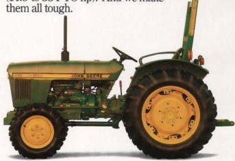
They've all got heavy-duty diesel engines and rugged sliding-gear transmissions. To keep them going strong year after year. They've also got differential lock and optional mechanical front-wheel drive to make the going easier on slopes, banks and other inconvenient places where grass thrives but tractors often fail.
