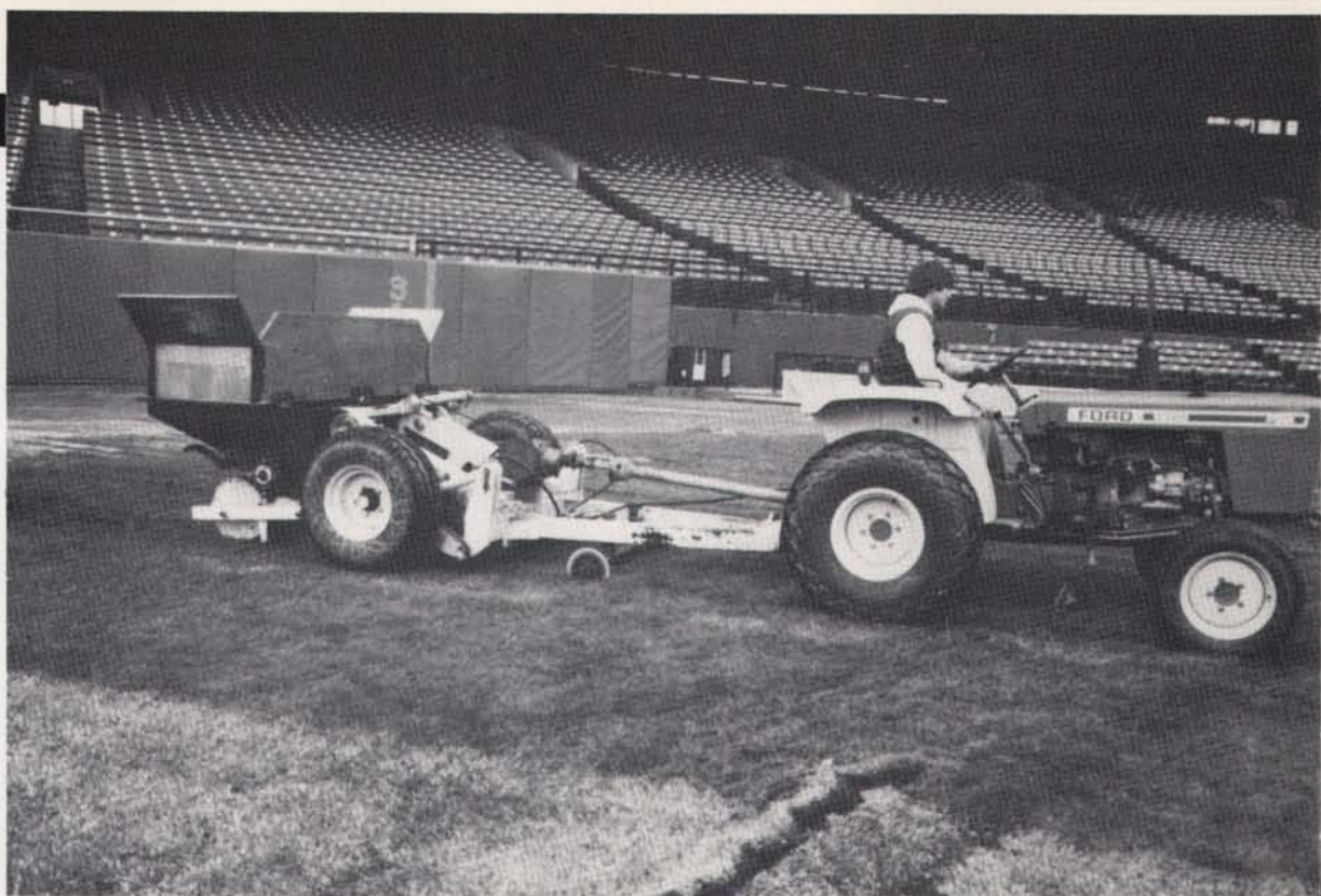
The sand groover, designed and used frequently in Europe, cuts and injects sand into two trenches at the same time.
