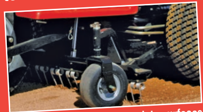
Spring Tine Scarifier chews into surfaces but skims over base spikes or pockets.
