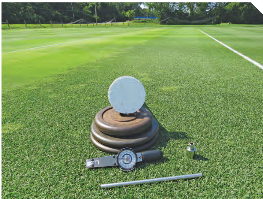
Traction apparatus used to measure the force (Nm) to initiate slip on grass courts. Apparatus disc was fitted with the soles from grass tennis shoes and weighted with 75 pounds. Peak force required to tear (break) the grass surface was then measured.
