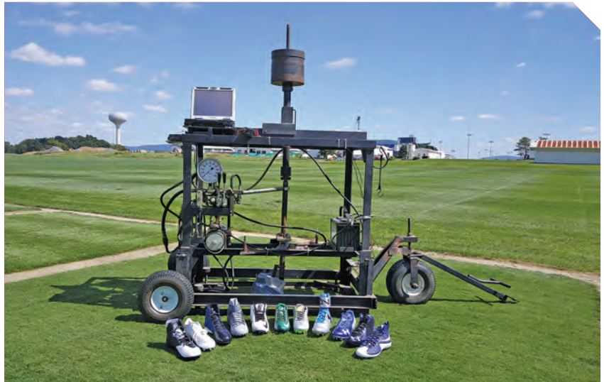
Penn State's Pennfoot measures rotational or translational traction.
