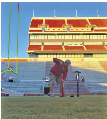
Clegg impact hardness measurement on the Oklahoma football field (photo courtesy of Jeff Salmond).
