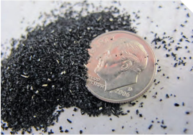
Comparable crumb rubber topdressing sizes. Photos courtesy of Kyley Dickson, PhD.
