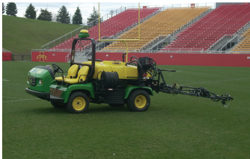
▲ The outside booms on this sprayer are each their own single zone and are automatically controlled by GPS. This doesn't allow any overlap and closely monitors flow rates and application rates from the operator's seat.
