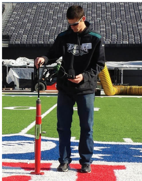
▲ Many field managers are now using a Clegg hammer to regularly measure Gmax on their own.
