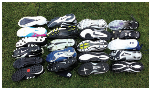
▲ The Center for Sports Surface Research recently measured rotational traction of 30 commercially available shoes on Kentucky bluegrass, bermudagrass, and FieldTurf Revolution. The difference among playing surfaces was minimal compared to the large differences found among shoes.
