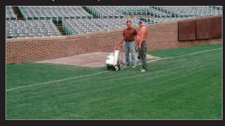
Roger O'Connor, left, former grounds crew leader for Wrigley Field, paints the field in 1984 using a type of paint striper. It uses a liquid propane tank (hopefully filled with compressed air and not propane) instead of a motor. It was silent and worked well, however it can lose pressure fairly quickly and need to be re-charged. If it was using LP gas, it would last much longer, but smoking near it was dangerous.
