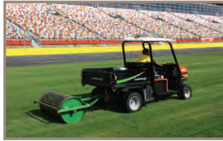
▲ Left: A grounds crew member repairs tire ruts left by school buses – yes, school buses. Charlotte Motor Speedway will race buses as part of its regular event schedule. Right: To help smooth out tire ruts and other irregularities, Pitts' crew uses a Cushman Turf-Truckster with a roller attachment.
